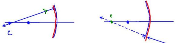
a ray through the centre of a curvature will reflect back along the same path
