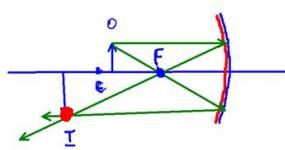
If the object is between the centre and the focus, the result is an inverted image that is real and large than the original
