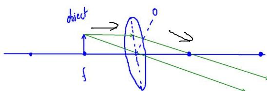
when the object is placed on  $f$  no image is produced
