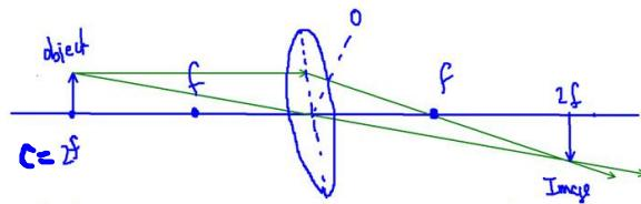
when an object is placed at  $2f$ , the image is inverted, same size as the object and real
