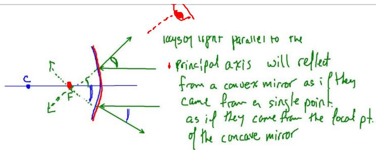
Light parallel to the principal axis will reflect from a convex mirror as if they came from a single point as if they come from the focal pt. of the concave mirror
