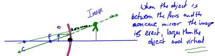
When the object is between the focus and the concave mirror the image is erect, larger than the object and virtual
