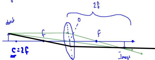
when an object is placed at a distance greater than  $2f$ , the image is inverted and smaller than the object and is real
