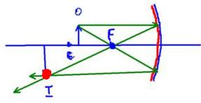
If the object is between the centre and the focus, the result is an inverted image that is real and larger than the original
