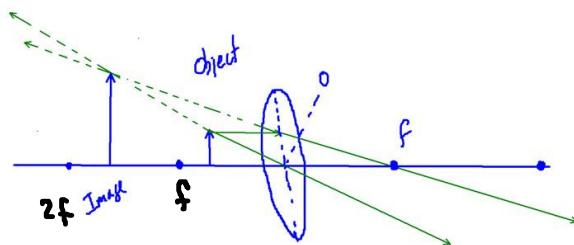
When an object is inside  $f$ , the image is erect, larger than the object and virtual
