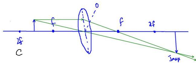
when an object is placed between  $f$  and  $2f$  the image is inverted, larger than the object and real
